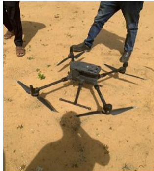
Photo 2: Drone DJI M300
